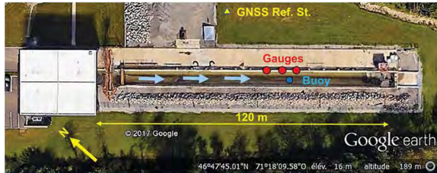
Figure 3. INRS hydraulic wave flume. Map data: Google, DigitalGlobe. [Colour online.]
