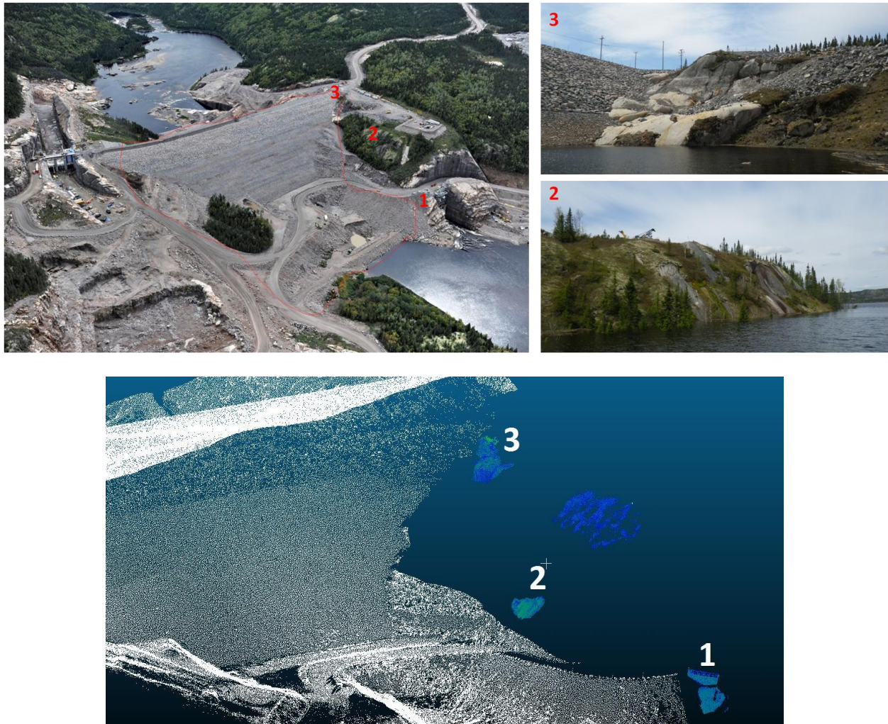
Figure 8: Reference LiDAR surfaces as defined by Hydro-Québec
